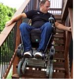
Here is a You Tube link to see how this I-bot can perform: <a href="https://youtu.be/O7otewMk9pc">https://youtu.be/O7otewMk9pc</a>. It really is cutting edge technology. Complete with gyroscopes for center of gravity, computerization for control and twin lighter weight lithium battery power packs. I-bots can go 6.5 mph and 17 miles! Other information is that the HVAMC is optimistically awaiting the "green light" to open its doors to volunteers. Please consider becoming a volunteer.
